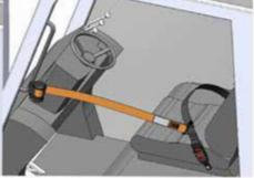
With safety belt engaged around wearer, EZE Retractor webbing stays taut and does not obstruct whilst manoeuvring the vehicle.
